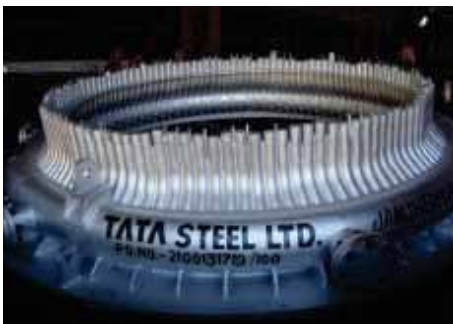
WATER COOLED HOOD (BOF)
