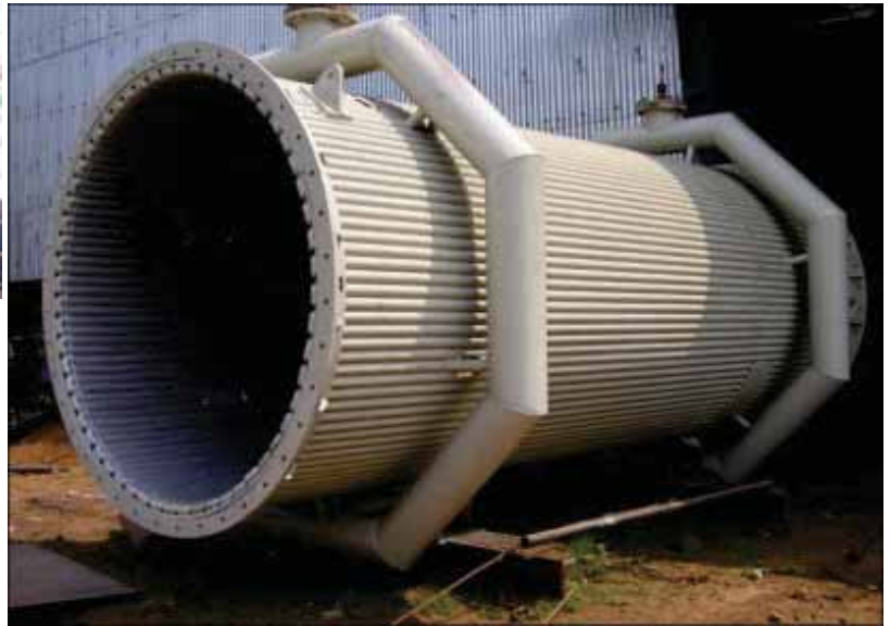
WATER COOLED DUCT
