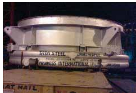
SKIRT WITH WATER COOLED COOLING
