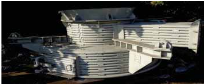
Ladle Furnace Roof at Prowess WORKSHOP
